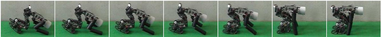
Figure 8: Dynamic phase III of getting up from the ground starting from the prone posture.
