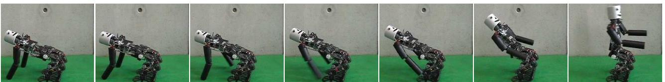
Figure 10: Dynamic phase III of getting up from the ground starting from the supine posture.
